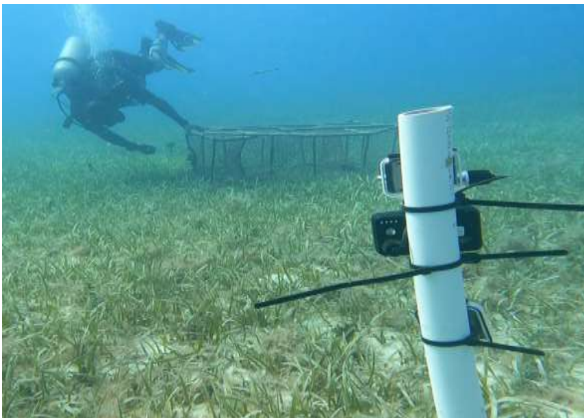
Figure 3. The non-harmful sampling station: which includes an underwater camera and an acoustic logger set in front of a Z-Antillean fish trap, and a camera inside of the trap. ©O'Sullivan & Cantor
