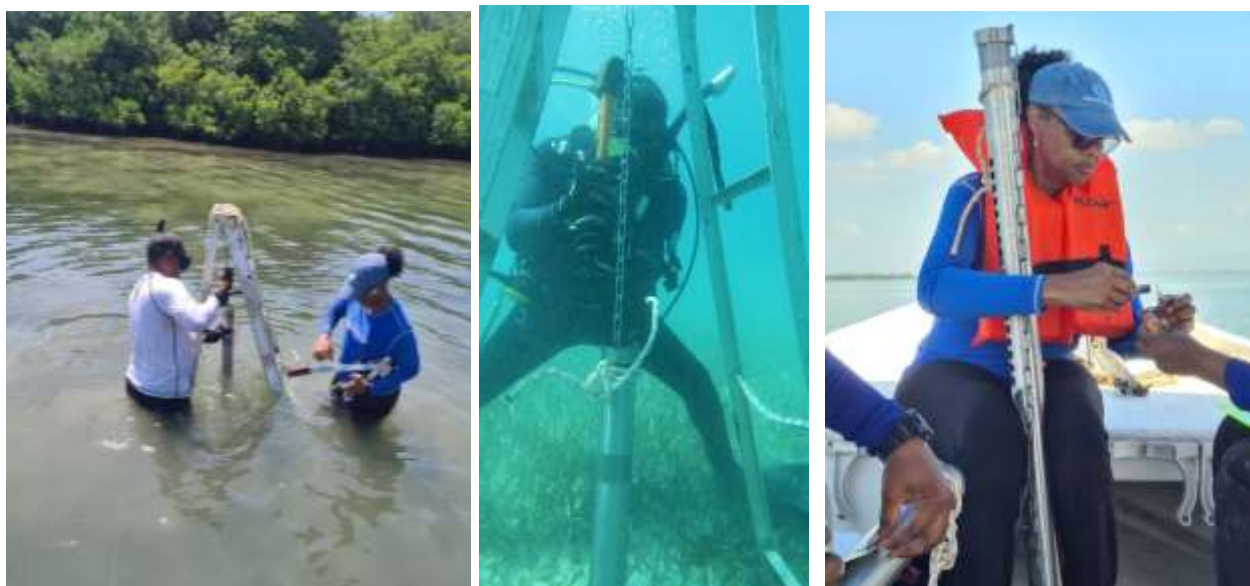
Figure 8. Deploying the CARICAS seagrass corer in the beds associated with Kingston Harbour mangroves (Left and Centre). Removing seagrass sediment sub-cores from the specially designed perforated seagrass corer (right).
